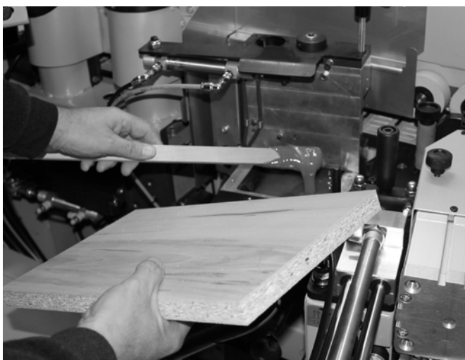
Fig. 10-9.1: Replacing the burnt glue
