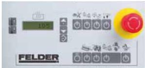
**1** Operating panel with LCD display and keypad
