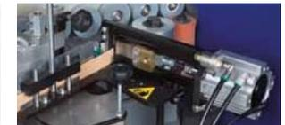
**6** Guillotine scissors - Pneumatic pre-sizing
