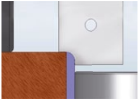
Radius trimming (R = 2 mm) from ABS/PVC- and veneer edges
