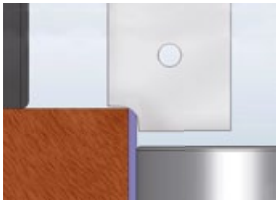
Bevel trimming of thin edges and coiled material (veneer)
